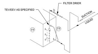
**4 TYPICAL DETAIL - PIPING DX UNIT WITH MAINS LOCATED ABOVE UNIT**
