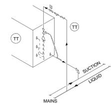
**3 TYPICAL DETAIL - PIPING DX UNIT WITH MAINS LOCATED BELOW UNIT**
